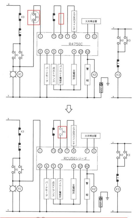
Mesure: Change Start contact to between terminal T1 & terminal T2.
