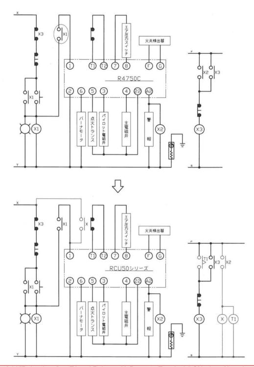
Mesure : Add "Delay timer" as T1 and Relay as X. Power to Terminal 1 ON when Alarm is generated.
