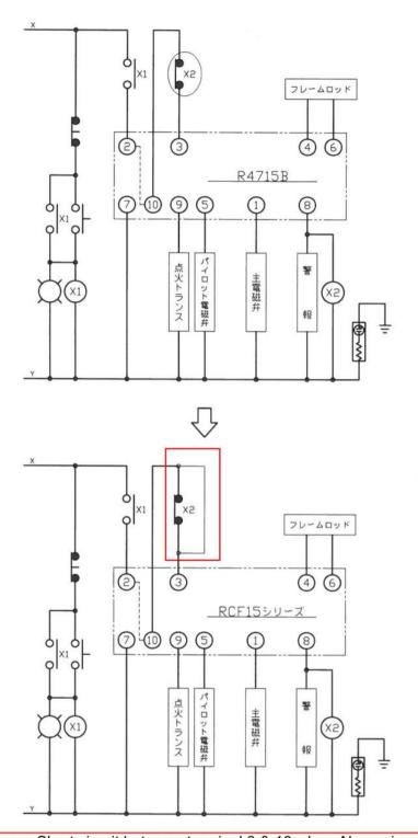
Mesure : Short circuit betwenn terminal 3 & 10 when Alarm signal is generetaed
