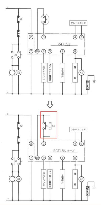
Mesure : Power ON betwenn terminal 3 & 10 when Alarm signal is generetaed
